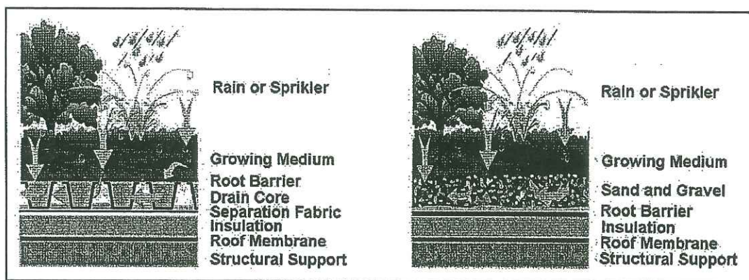
Figure B.3 – Green Roof Profile
