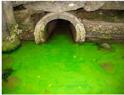
Dye in the Marine Water from an OSS with a Broken Transport Line
