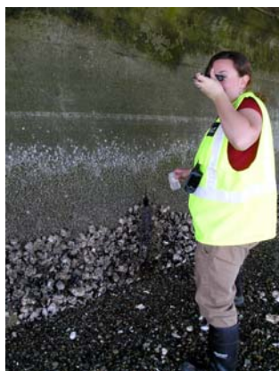
Using a Refractometer to Determine Salinity
